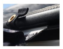
2. Take the awning piping and slide it through the caravan awning channel, until the awning is in the desired position on the vehicle; we recommend someone else holding the flysheet up whilst you do this.
